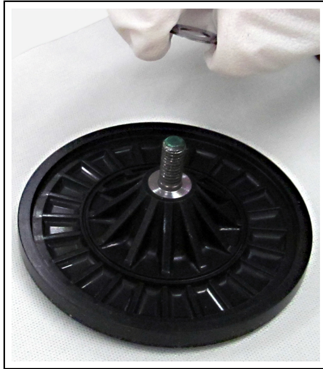
Figure 7-11 Placing original spacers on new diaphragm
